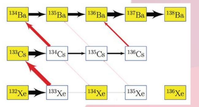
Figure 9: Publication no. 125 - The s-process path at the vicinity of <sup>134</sup>Cs at T = 0.35 GK (kT = 30 keV) generated by the NUCNET code (Bojazi & Meyer 2014). The red lines present  $\beta$ -decay, while the black lines present the neutron capture. Line width indicates the flow current in linear scale. The stable nuclei are marked with yellow color.
