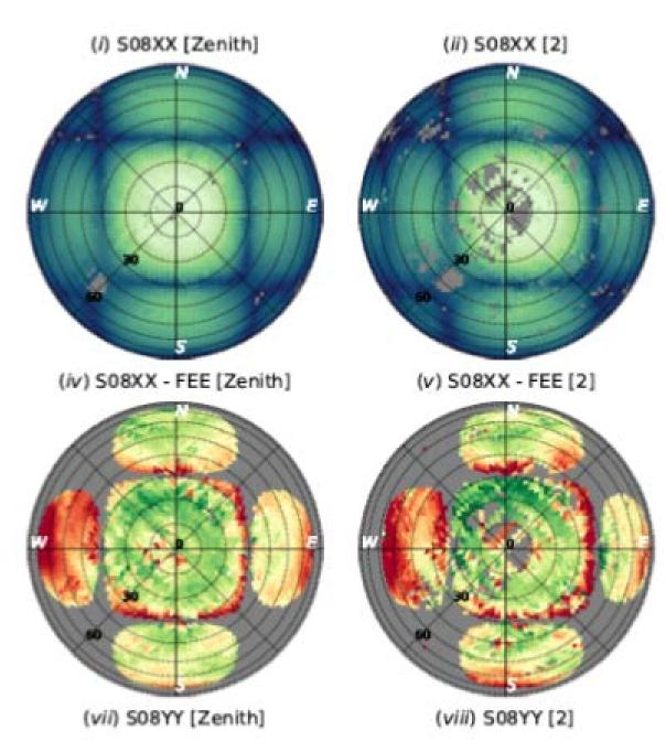
Figure 8: MWA primary beam sky response, mapped via passes over the array of an Orbcomm satellite (top), and difference compared with model (bottom). Chokshi et al 2021, "Dual Polarization Measurements of MWA Beampatterns at 137 MHz", Monthly Notices of the Royal Astronomical Society, Volume 502, Issue 2, pp.1990-2004
